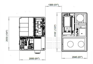
Machine layout shows the max. size of COOLPULSE<sup>TM</sup> Unit which can differentiate from final layout.
