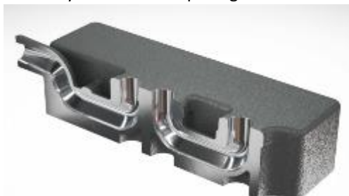
Above: Media flowing through the internal passages Below: shiny clean internal passages after AFM
