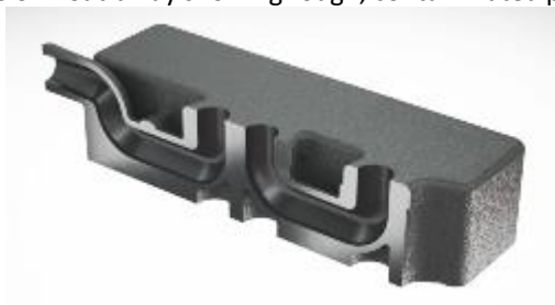
Above: 3D Printed manifolds including organic channels Below: Cut-away showing rough, contaminated passages
