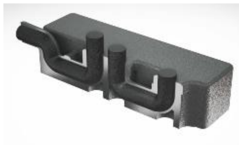
Above: Media flowing through the internal passages Below: shiny clean internal passages after AFM
