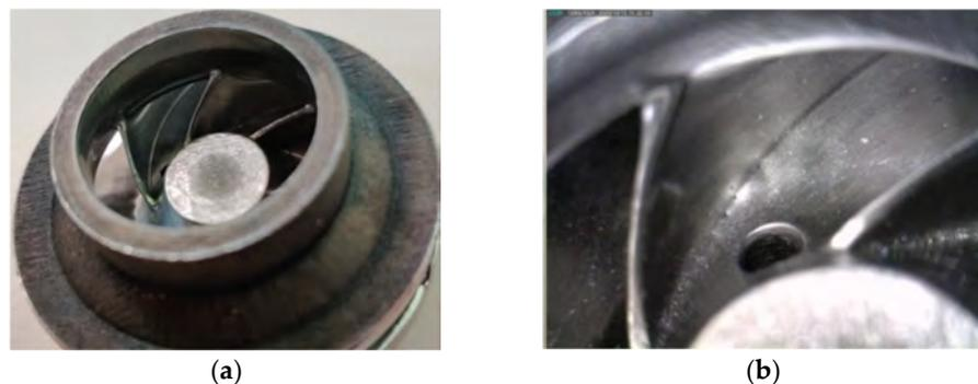
**Figure 11.** Images presenting the (a) closed impeller after AFM process and (b) close view of the finishing process.
