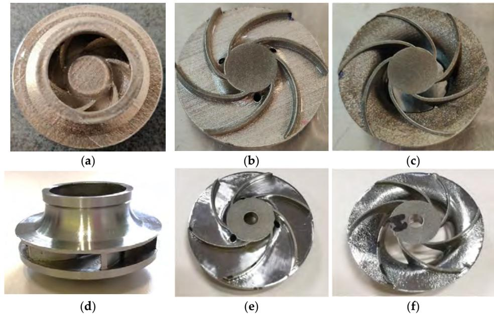
**Figure 12.** Post-processed (turned) closed impeller: (a) as-printed closed impeller; (b) as-printed disc half; (c) As-printed shroud half; (d) finished closed impeller; (e) finished disc half; (f) finished shroud half.
